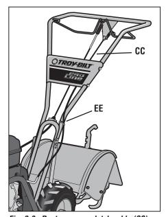
Fig. 2-9: Route reverse clutch cable (CC) as shown. Attach to handlebar with cable tie (EE).
